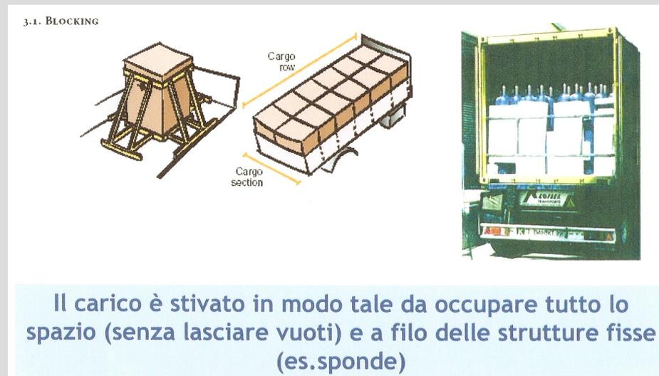
PER IL RIEMPIMENTO DEGLI SPAZI VUOTI POSSONO ESSERE UTILIZZATI H-BLOCK, ZEPPE, PALLET, AIRBAG, ECC.
